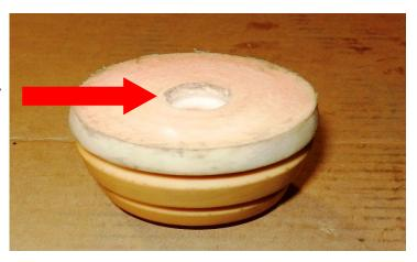
Use a soap and water solution to aid in installation, push the bump stops into the ReadyLIFT extensions with a twisting motion. Make sure they fully seat.
