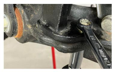
Reinstall the factory torsion bars and torsion keys. Make sure the torsion bars are installed in the same direction as they were installed from the factory. Leave the torsion keys loose. Do not add the cross pin or set screw at this time. Add the new torsion bar bracket to the torsion bars.
