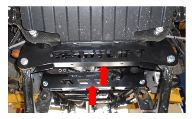
Install the lower control arms to the ReadyLIFT cross members using the provided M18 bolts, washers, and nuts. Do not tighten at this time.
