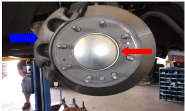
Remove the axle nut and brake rotor.
