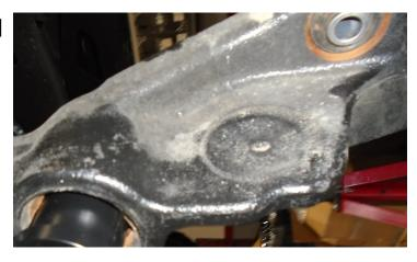
Install the 7/16" bolt, washer, and top lock nut. Torque to 55 ft-lbs.
