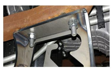
Install the ReadyLIFT driver side diff drop to the diff cradle using provided M12 bolts and washers to the forward two locations. Install the last mount using the factory bolt and a provided M12 washer and nut. Do not tighten at this time.
