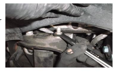
Measure and record the torsion key adjuster bolt length. Remove the torsion bar adjustment bolt.
