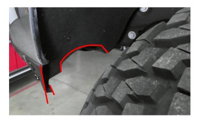
Remove the front wheel mud flap. mark a straight horizonal line 2" from the seamed edge. Use a suitable cutting tool, cut along the marked edge. Reinstall the mud flap.
