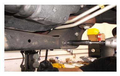
Disconnect the electrical connectors and vent tube from the differential.
