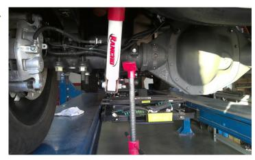
Loosen but do not remove the U-bolts one the side of the axle. This will allow slack. With a suitable jack remove the U-bolts on the opposite side and discard.
