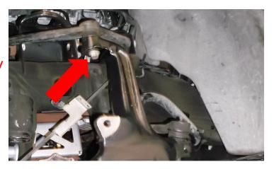
Install the hub assembly and dust shield to the ReadyLIFT knuckle using the factory hardware and a drop of thread locker. Torque to 120 ft-lbs.
