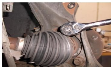
Support the LCA with a suitable jack. Loosen but do not remove the upper and lower ball joint nuts. Strike the ball joint boss on the knuckle to dislodge the tapers. Remove the knuckle from the upper and lower control arms.
