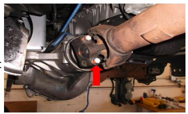
Install the ReadyLIFT front and rear cross member. Use the factory control arm and cross member hardware. Do not tighten at this time.
