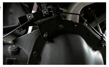
Remove the factory rear shocks. Retain hardware.
