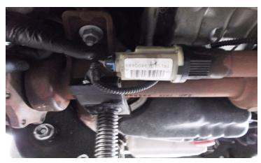
Mark the front drive shaft to pinion orientation for reinstallation later. Remove the front drive shaft from the differential. Let hang out of the way.
