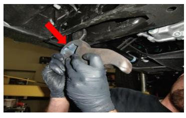
Loosen but do not remove the outer tie rod end nut at the knuckle. Strike the tie rod boss with a dead blow hammer to dislodge the taper. Remove the tie rod after this has been completed.
