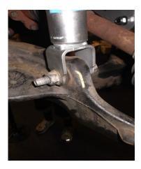
Install the outer tie rod ends to the ReadyLIFT knuckles using the factory hardware. Torque to 65 ft-lbs.
