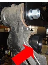
Mark the front side only of the transmission cross member where the torsion bars pass through. Mark at the 1 o'clock position and 5 o'clock position draw a 1/4" thick clearance line between these marks.
