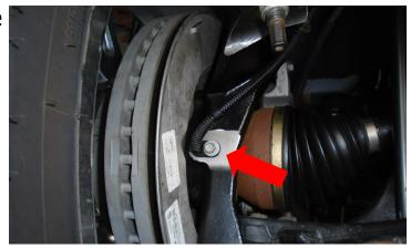
Attach the ABS wire bracket to the top hole on the knuckle. Use factory hardware. Attach the brake line and ABS wires to the provided bracket. Use supplied hardware. Attach the new bracket to the lower mount on the knuckle.
