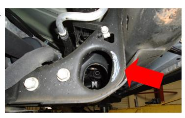
Using a suitable cutting tool, cut along the previous made marks. Remove and discard the outer portion of the cross member. Paint the exposed metal with a quality rust preventative paint.
