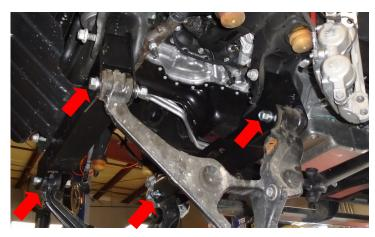
Tighten and torque the ReadyLIFT cross members to the frame. Torque to 150 FT-LBS. Do not tighten the LCA these have bonded bushings and must be tightened when the vehicle is at ride height.
