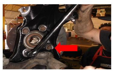
Reinstall The CV axle. Make sure to line up the previous marks on the flanges.
