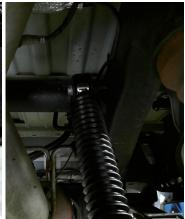
Install the provided brake line bracket to the differential. Use factory hardware. Attach the brake line to the extended bracket. Use provided hardware. Torque to 20 ft-lbs.
