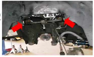
Remove the front two driver/ passenger LCA bump stops from the frame. You may need to smack them with a dead blow hammer to dislodge them. Be careful of the rebound. Retain factory bump stops. Do not remove the rear bump stop.
