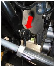
Remove the axle dust cover using a chisel or other suitable tool. Remove the brake caliper from the knuckle. Use a suitable device and hang the caliper out of the way. DO NOT let the caliper hang by the rubber brake line.
