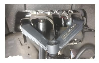
Raise the lower control arm up and support with a suitable stand. Install the ReadyLIFT knuckle to the lower and upper ball joint using the factory nuts. Torque the upper ball joint to 65 ft-lbs, and the lower ball joint to 85 ft-lbs. Transfer the o-ring from the inside of the factory knuckle to the ReadyLIFT knuckle.
