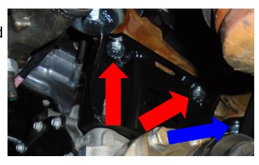
Raise the diff up to its new mounting location. Attach the passenger side bracket to the diff. Use the provided M12 bolts, washers and factory nuts.
