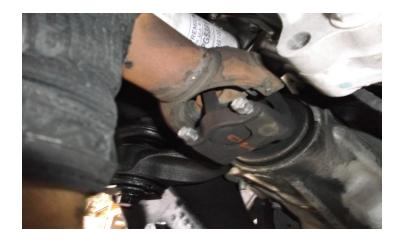
Support the differential with a suitable jack / stands, remove the driver and passenger side hardware. Mark the hardware locations as the bolts must be reinstalled in specific spots. Carefully lower the differential out of the vehicle and set aside.
