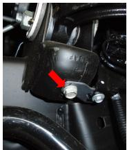
Remove the sway bar end links from the LCA and the sway bar. Discard the end links and hardware.
