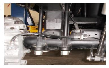
Install the provided U-bolts and nuts. Snug up but do not tighten at this time. Repeat for the opposite side. When tightening, use a criss-cross pattern. Alternate between sides of the vehicle. Final torque will be completed when the vehicle is on the ground.
