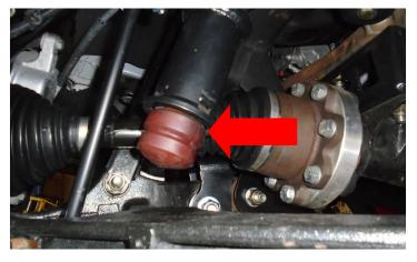
Reinstall The CV axle factory nut. Torque to 165 ft-lbs.
