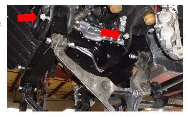
Install the provided torsion bar bracket spacer into the torsion bar pocket on the lower control arm. Install the spacer from the back side of the LCA and add the collar to the spacer from the front side of the LCA
