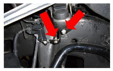
Attach the wheel speed sensor to the steering knuckle. Use factory hardware. Torque to 10 ft-lbs.
