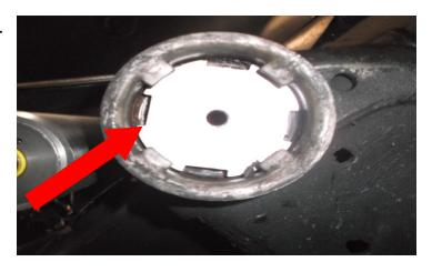
Place the ReadyLift Bump Stop Extension Washer between the bump stop and vehicle. Install the Ready-LIFT bump stop extension using provided 3/8" x 5.5" long Allen head bolt and washer. Torque to 35 ft-lbs.
