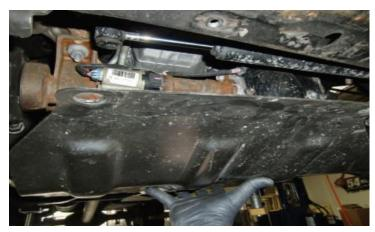
Remove the shock hardware from the frame and lower control arms (LCA). Discard the shocks and upper shock hardware. Retain the LCA shock hardware.
