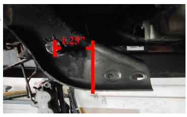
Using a suitable cutting tool, cut along the previous made marks. Remove and discard the outer portion of the control arm pocket. Paint the exposed metal with a quality rust preventative paint.
