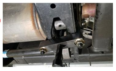
Install factory adjustment bolt. Set the bolt to the recorded Measurement from page 7.
