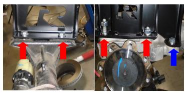
Torque all diff hardware 95 ft-lbs starting with the driver and passenger side upper hardware first. Then driver lower hardware. When tightening the passenger side lower hardware, makes sure to "center" the bracket in the diff's slotted mount. Verify that the diff clears the frame cut made earlier. If not, trim more frame material out until a minimum 1/4" clearance is gained. The frame should rest right inside the divot in the diff housing between the middle and last bolt bosses.
