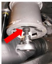
Take the factory bump stops and grind the top edge at a slight angle to aid in installation later. Drill out the top of the bump stop with a 1/2" drill bit 3/4" deep.
